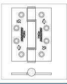
4720 – 110x98mm Offset Lift Off Hinge (handed) Grade 304 stainless steel or CS4 mild steel EN 1935:2002 Grade 13 CE Certificate Nos. 1121-CPD-AC0084/AC0086/AC0069 Certifire 30min and 60min Assessment Report CF769 Warrington Fire Assessment Report 30min and 60min WFAR176781 Fire tested in accordance with EN 1634-1:2000 and CE Marked Supplied with No. 10 11/4" screws Maximum adjusted door weight: 120kg Recommended minimum door thickness: 44mm
